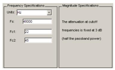
After specifying the filter design parameters, click the **Design Filter** button at the bottom of the design panel to compute the filter coefficients. The display updates to show the magnitude response of the designed filter.
